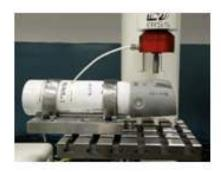
BISS Low Force Systems (LFS) cover the needs of practically any mechanical test on materials and subcomponents. They reflect over three decades of innovation, research and worldwide experience in servotest technology. LFS are ideal for testing of miniature material specimens, micro-electronic connections and subcomponents, biomaterial (tissue engineering) and much more.
