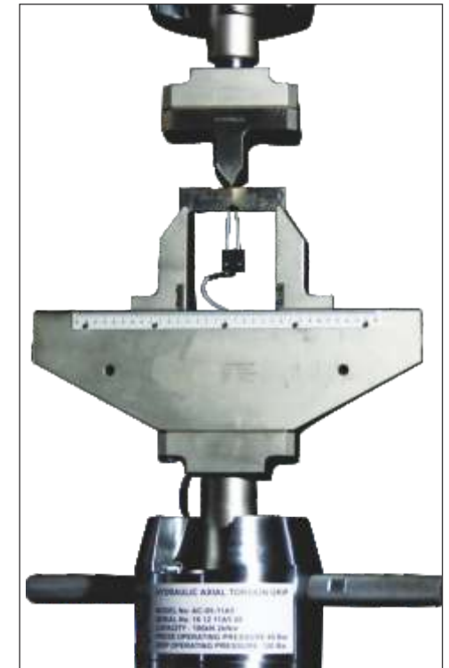
Three Point Bend Grips for SE(B) specimen with COD Gage
