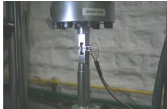
Fatigue crack propagation test using DCPD unit
