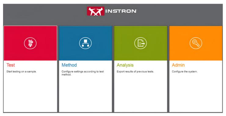
Test Builder Application Software with its most intuitive workflows is designed to suit static, monotonic and user defined fatigue cycling testing. It is designed to help increase testing efficiency and minimize safety hazards. The home screen of the application software has been categorized into 4 major tabs namely the Test, Method, Analysis and the Admin tab to help user identify the relevant section to be accessed when in operation.
