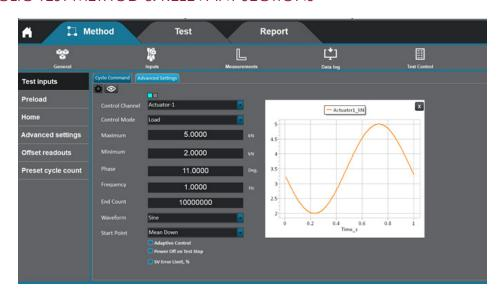
All systems at Instron are built considering safety achievable to the highest level. A dedicated section in the methods tab helps set up the upper and lower safety limits for stoke, load and strain channels to trip, hold or stop the test when in emergency or uncontrolled occurrence of any event.
